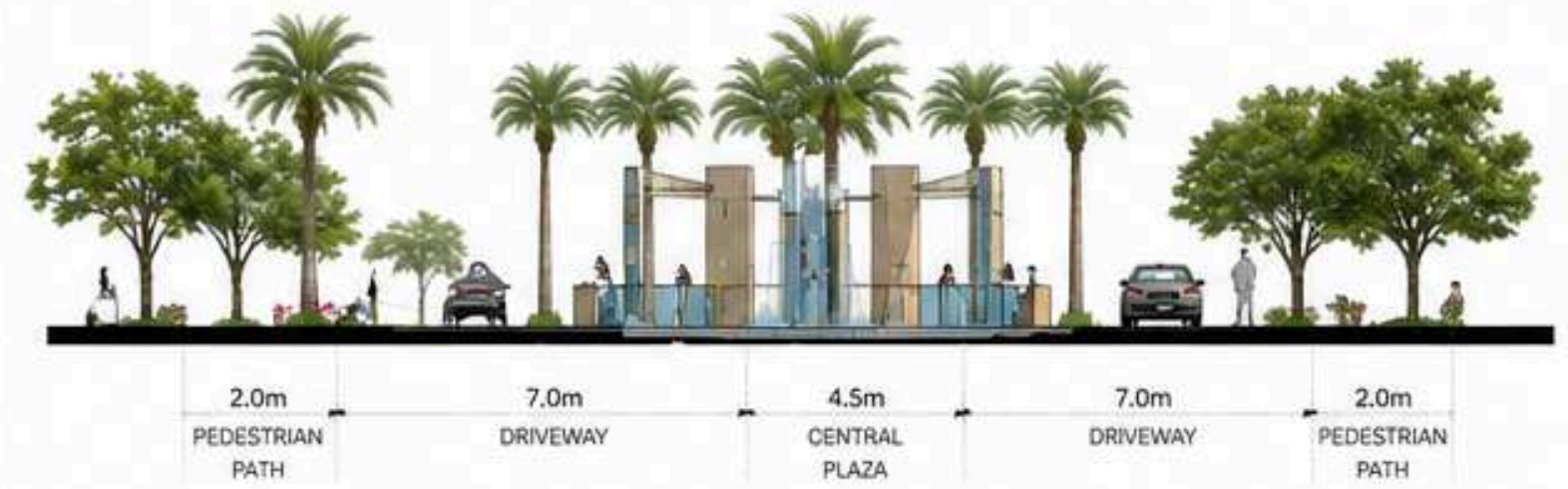
Section A-A' Illustrating spatial organisation of central median, circulation, and landscape layering.
